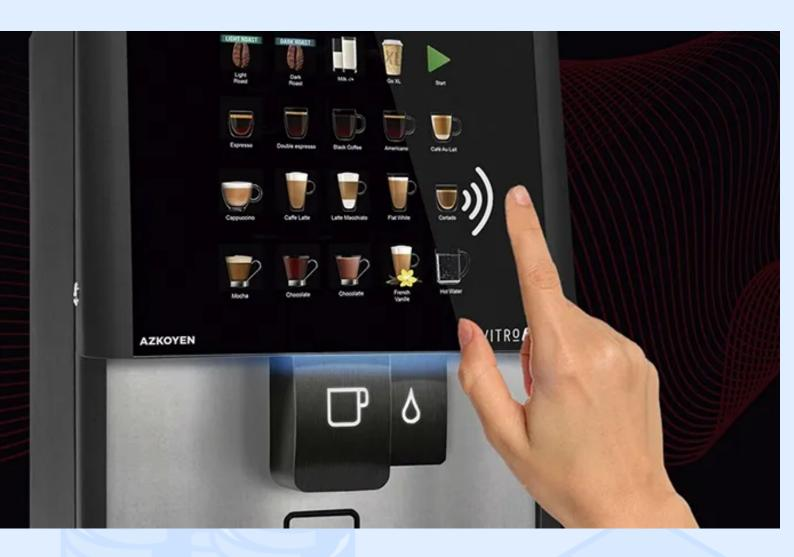
New contactless machines have appeared in coffee retail. For example, Azkoyen Group's Air Touch technology allows devices to make product choices without touching the screen. The system will determine the user's choice at a distance of a couple of centimetres, which means that now self-service will also become hygienically safe.
