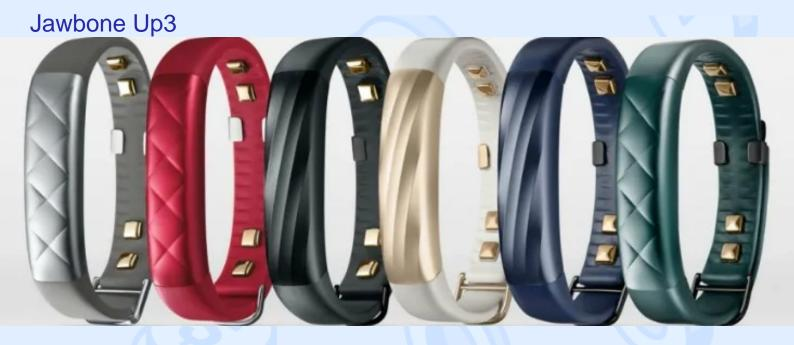
Jawbone Up3 is built on a sophisticated multi-sensor platform that packs in an innovative tri-axis accelerometer, bio-impedance sensors, as well as a galvanic skin response and temperature sensors. No wonder that the device is advertised as "the most advanced activity tracker known to man" - thanks to these multiple sensors, it can measure resting and passive heart rate to provide its wearers with a holistic view of their heart.
