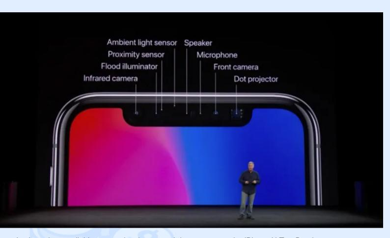
Apple makes available to app developers real-time access to the iPhone X TrueDepth camera system. It is now possible to implement visual effects and user interactions based on a 3D scene from the camera.
