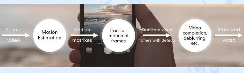
Let's describe the process in detail. Video stabilisation is achieved by first estimating the interframe motion of adjacent frames. At the end of this step we have the array of matrices 3×3, each of them describes the motion of the two adjacent frames. The accuracy of the global motion estimation is crucial as the first step of the stabilisation.
